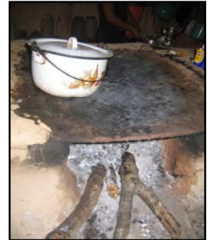
Plancha and exposed burning chamber
